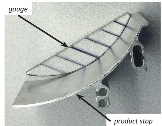
**Figure 3.** The product stop shown here is good. It conforms with the curve of the gauge.
