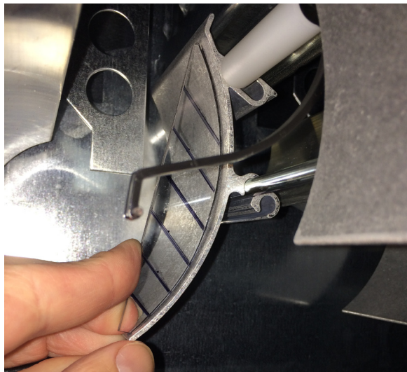
Figure 3. The product stop shown here is good. It conforms with the curve of the gauge.
