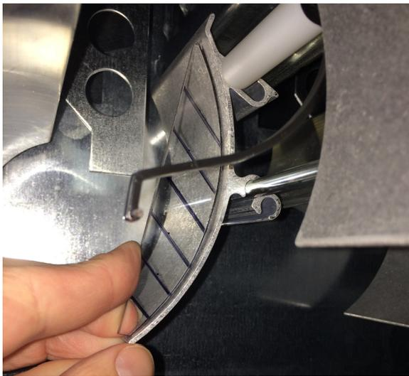
**Figure 2.** The product stop shown here is good. It conforms with the curve of the gauge. (Shown outside the vender in this photograph for clarity.)
