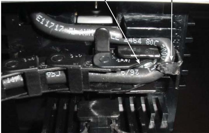
**Figure 10.** Attach the end of the elevator cup assembly harness to the chain adapter bracket.
